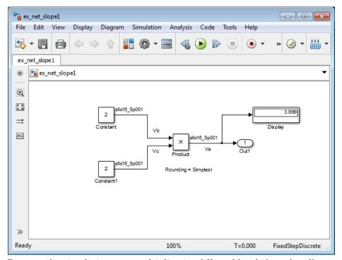
Because the simulation uses multiplication followed by shifts to handle the net slope correction, net slope precision loss occurs. This precision loss results in numerical inaccuracy: the calculated product is 3.999, not 4, as you expect.
