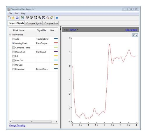
The preceding plot of the plant output signal reflects the initial guess at scaling. The Bode plot design sought to produce a well-behaved linear response for the closed-loop system. Clearly, the response is nonlinear. Significant quantization effects cause the nonlinear features. An important part of fixed-point design is finding a scaling that reduces quantization effects to acceptable levels.
