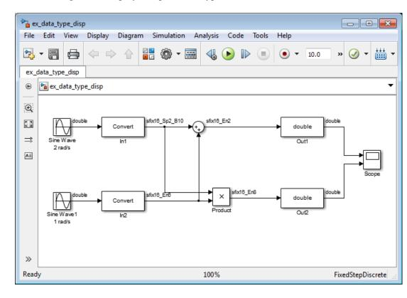
In the model, the data type displayed with the In1 block indicates that the output data type name is sfix16\_Sp2\_B10. This corresponds to fixdt(1, 16, 0.2, 10) which is a signed 16 bit fixed-point number with slope 0.2 and bias 10.0. The data type displayed with the In2 block indicates that the output data type name is sfix16\_En6. This corresponds to fixdt(1, 16, 6) which is a signed 16 bit fixed-point number with fraction length of 6.
