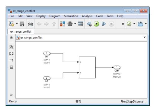
The model uses block annotations to display the specified design minimum and maximum values for the blocks in the model.
