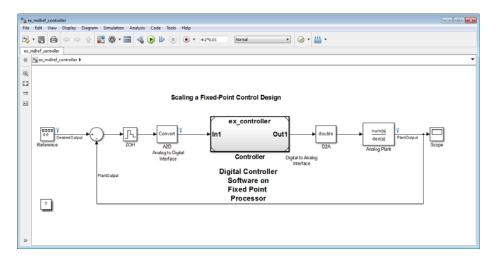
The model contains a Model block that references the ex controller model. Using a referenced model isolates the controller from the rest of the system. This method is useful to help you configure a model to determine the effect of fixed-point data types on a system. Using this approach, you convert only the referenced model because this is the system of interest.
