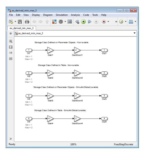
The model uses block annotations to display the specified design minimum and maximum values for the Inport blocks. The design range for all Inport blocks is [1,2].
