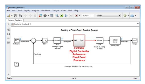
The Simulink model of the feedback design consists of the following blocks and subsystems:
