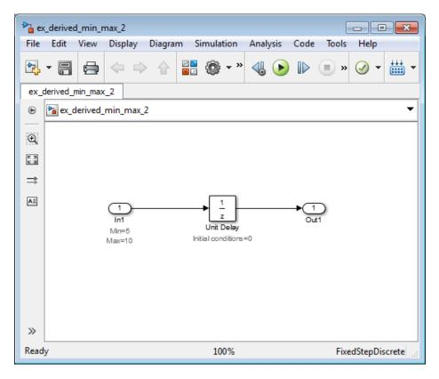
The model uses block annotations to display the specified design minimum and maximum values for the Inport block and the initial conditions for the Unit Delay block.
