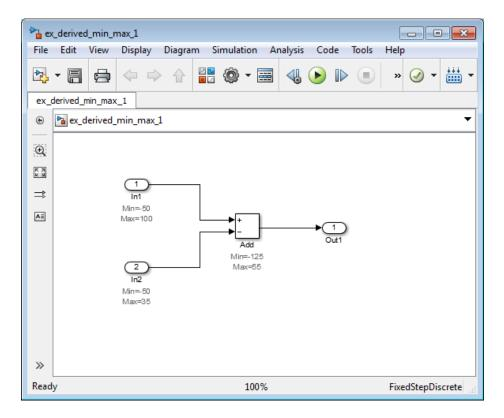
The model uses block annotations to display the specified design minimum and maximum values for each block.
