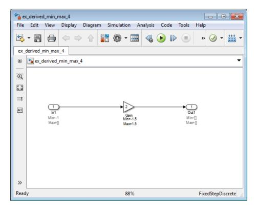
The model uses block annotations to display the specified design minimum and maximum values for the blocks in the model.
