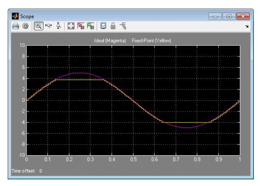
The Scope displays the real-world and fixed-point simulation results.
