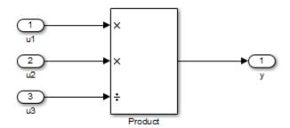
As stated in the C standard, the most efficient rounding mode for multiplication operations is always floor. However, the C standard does not specify the rounding mode for division in cases where at least one of the operands is negative. Therefore, the most efficient rounding mode for a divide operation with signed data types can be floor or zero, depending on your production target.
