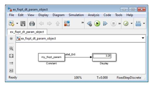
Consequently, the Constant block outputs a signed fixed-point value of 3.3, with a word length of 8 bits and a fraction length of 3 bits.
