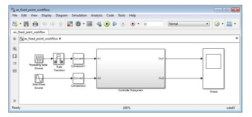
The model consists of a Source, a Controller Subsystem that you want to convert to fixed point, and a Scope to visualize the subsystem outputs. This method is how you configure a model to determine the effect of fixed-point data types on a system. Using this approach, you convert only the subsystem because this is the system of interest. There is no need to convert the Source or Scope to fixed point.
