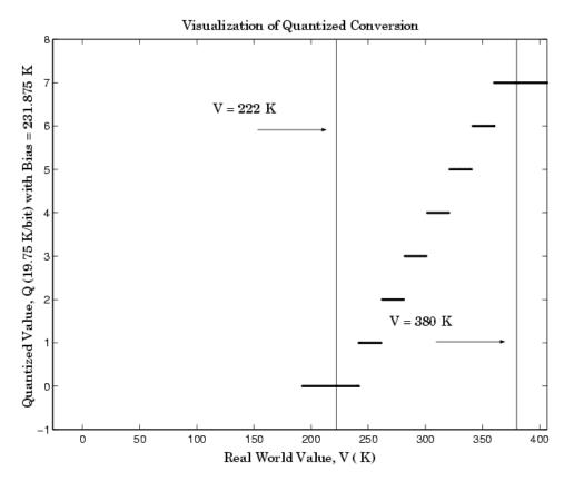
The quantization error is -9.875 K/bit  $\leq Error \leq 9.875$  K/bit, which is approximately 2.5 times smaller than the error associated with the purely linear conversion.
