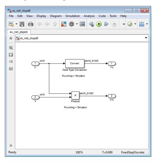
In this model, the net slope for the Data Type Conversion and Product blocks is 1/1000.
