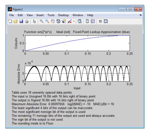
The upper plot shows the ideal function  $\sin(2\pi x)$  and the fixed-point lookup approximation between the breakpoints. In this example, the ideal function and the approximation are so close together that the two graphs appear to coincide. The lower plot displays the errors.
