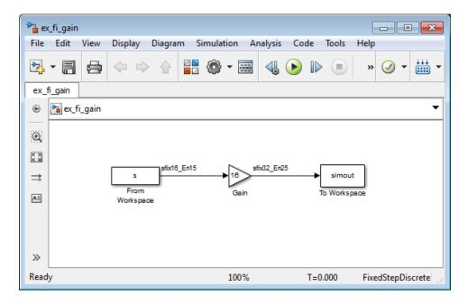
The To Workspace block writes the result of the simulation to the MATLAB workspace as a fi structure.
