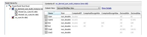
If a model contains multiple instances of the referenced model, the tool displays each instance of the referenced model as well as a node for the referenced model. For example, here are the results for the first instance of the referenced model ex sum1 in ex multi instance.
