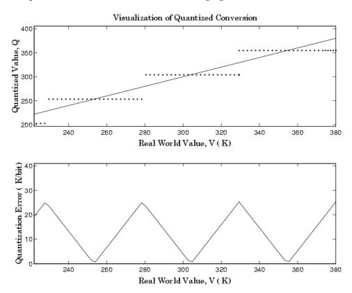
As an alternative to the purely linear conversion, consider the general linear conversion with maximum precision:
