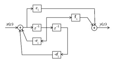
$$\frac{y(z)}{x(z)} = \frac{e_i + f_i z^{-1}}{1 + c_i z^{-1} + d_i z^{-2}}$$
