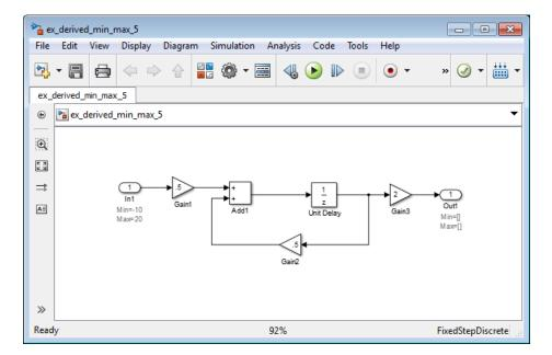
The model uses block annotations to display the specified design minimum and maximum values for the blocks in the model.
