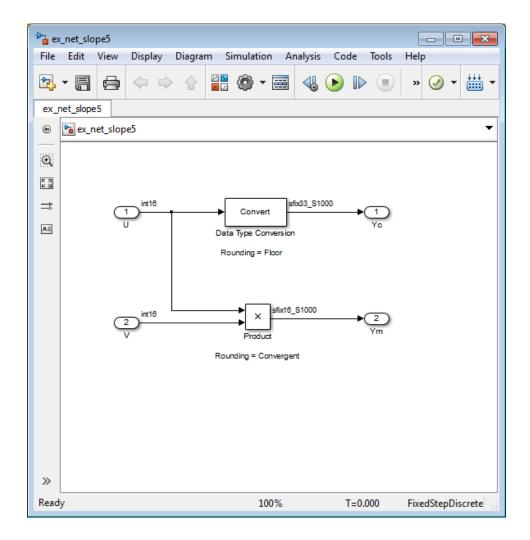
In this model, the net slope for the Data Type Conversion and Product blocks is 1/1000.
