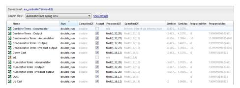
6 Review the scaling that the Fixed-Point Tool proposes. You can choose to accept the scaling proposal for each block by selecting the corresponding **Accept** check box in the **Contents** pane. By default, the Fixed-Point Tool accepts all scaling proposals that differ from the current scaling. For this example, verify that the **Accept** check box associated with the active run is selected for each of the Controller subsystem's blocks.
