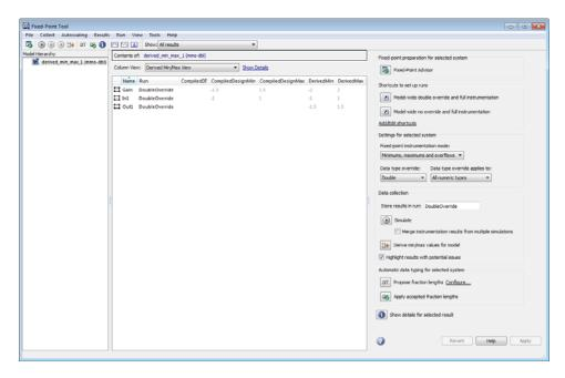
If the analysis cannot derive a minimum or maximum value, the Fixed-Point Tool highlights the result. To fix the issue, examine the model to identify which objects have no specified design ranges and add this information. See "Insufficient Design Range Information" on page 10-20.
