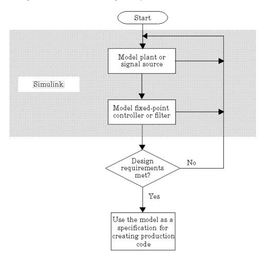
Using the MATLAB, Simulink, and Simulink Fixed Point software, you follow these steps of the development cycle:
